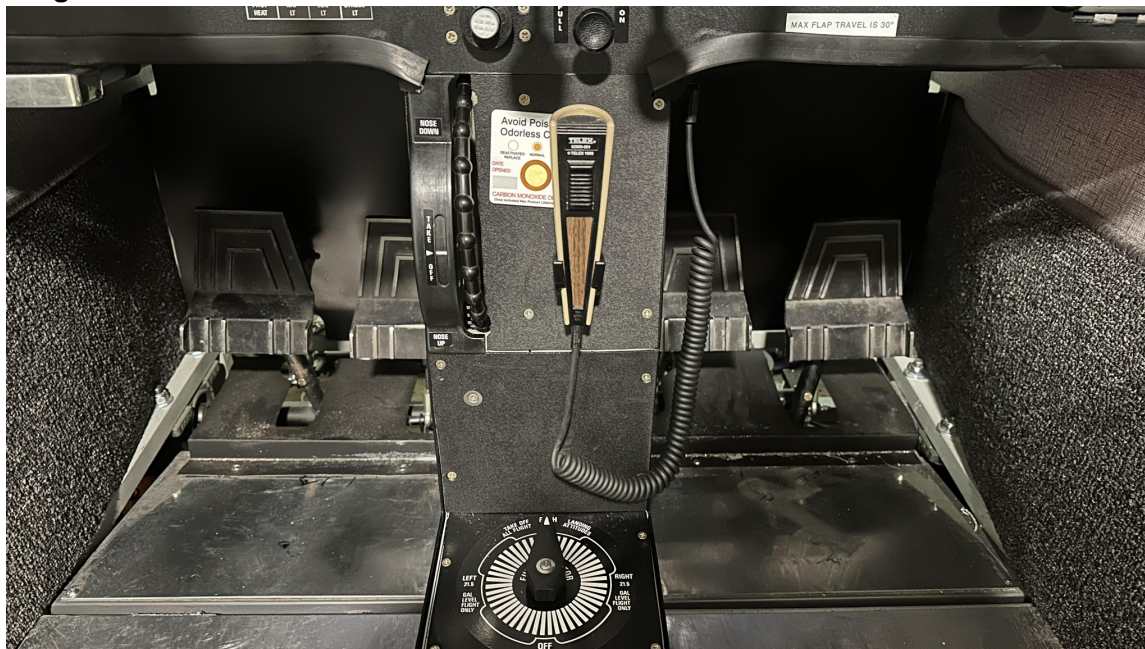
Image 10. Rudder Pedals, Trim Wheel, Trim Indicator and Fuel Selector
