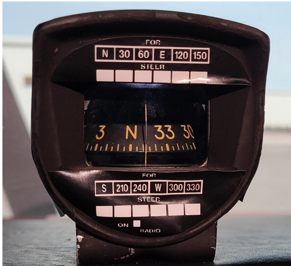
Image 3. Detailed view of the mechanical compass
