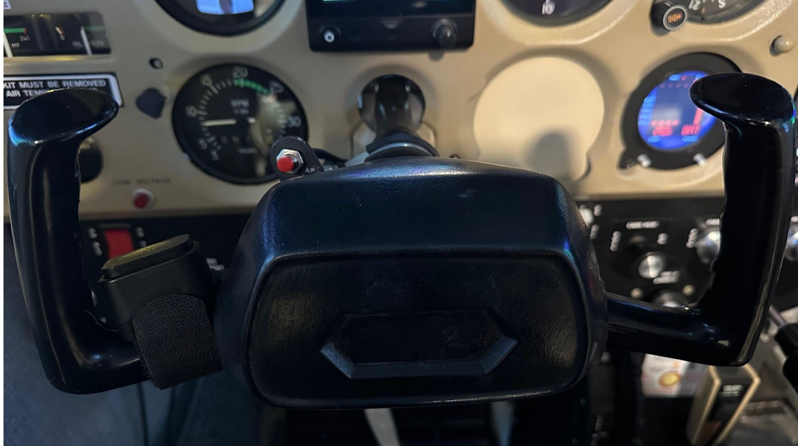
Image 7. Yoke mounted switches (A/P disengage and PTT)
