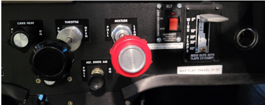
Image 9. Engine controls and Flap Selector/Indicator
